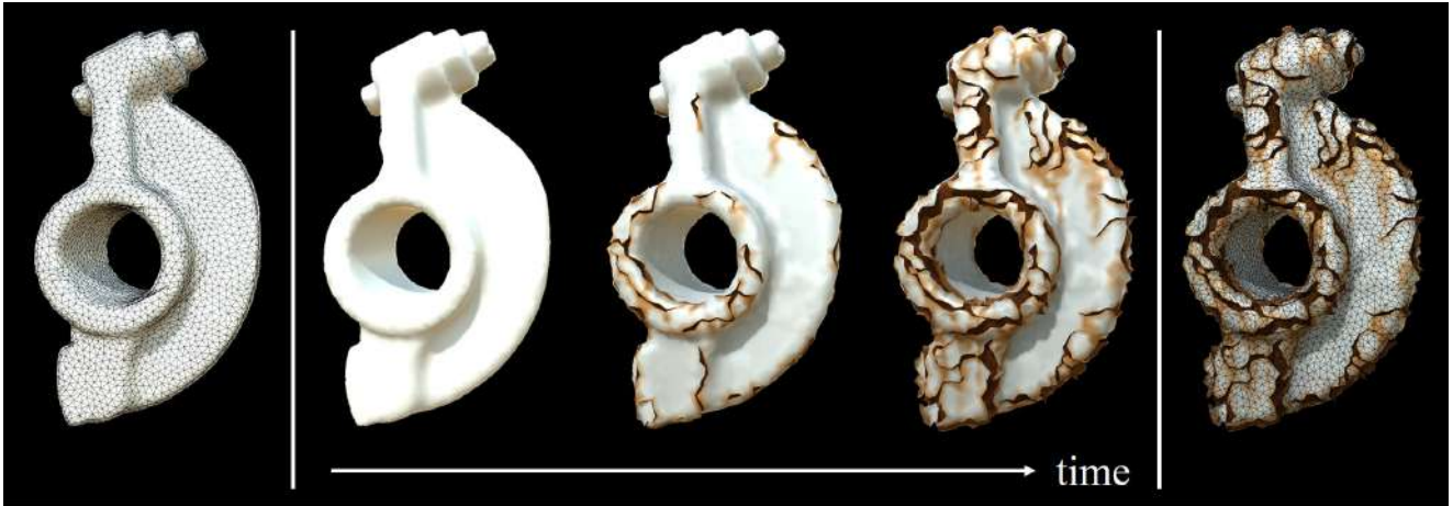
Fig. 1: Deterioration process of a mechanical part, simulated using the proposed method. The left- and right-most show the initial and final states of the mesh, respectively. The method does not deal with remeshing during the simulation, but it can generate cracks naturally by targeting a model with a uniformly random triangle mesh
